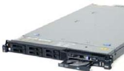
The x3550 M2 contains **six** drive bays in all. Hot-swap drives may be inserted or removed through the front of the server without powering off the system. Simple-swap solid-state drives can be inserted or removed through the front of the server as well; however, the system power must first be turned off.
